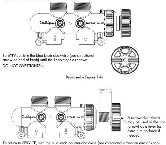
To return to SERVICE, turn the blue knob counter-clockwise (see directional arrow on end of knob) until the knob stops as shown. DO NOT OVERTIGHTEN!
