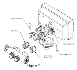
**Note:** The bypass stem can only be removed from valve on the bypass side (red knob). The bypass valve is designed so that it can be flipped over, with the bypass (red) knob on the left side of the valve. This will need to be taken into consideration if the control is plumbed in close to a wall which may prevent the stem from being easily removed.
